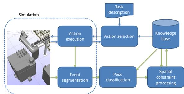
Fig. 1: Spatial constraints embedded in an action selection system. The spatial constraints are solely based on pose and object type information, feeding relevant contextual information to an action selection module that may choose actions variants based on the spatial constraints.
